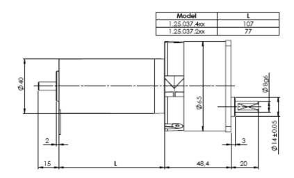
Note: Pole (+): left side, view output shaft.
